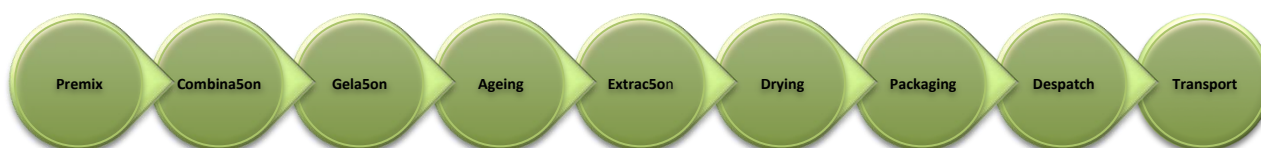
Spaceloft Production Process
