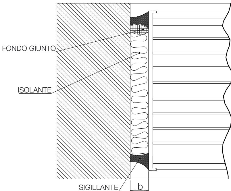
Minimum junction width "b" for injected insulator substance
